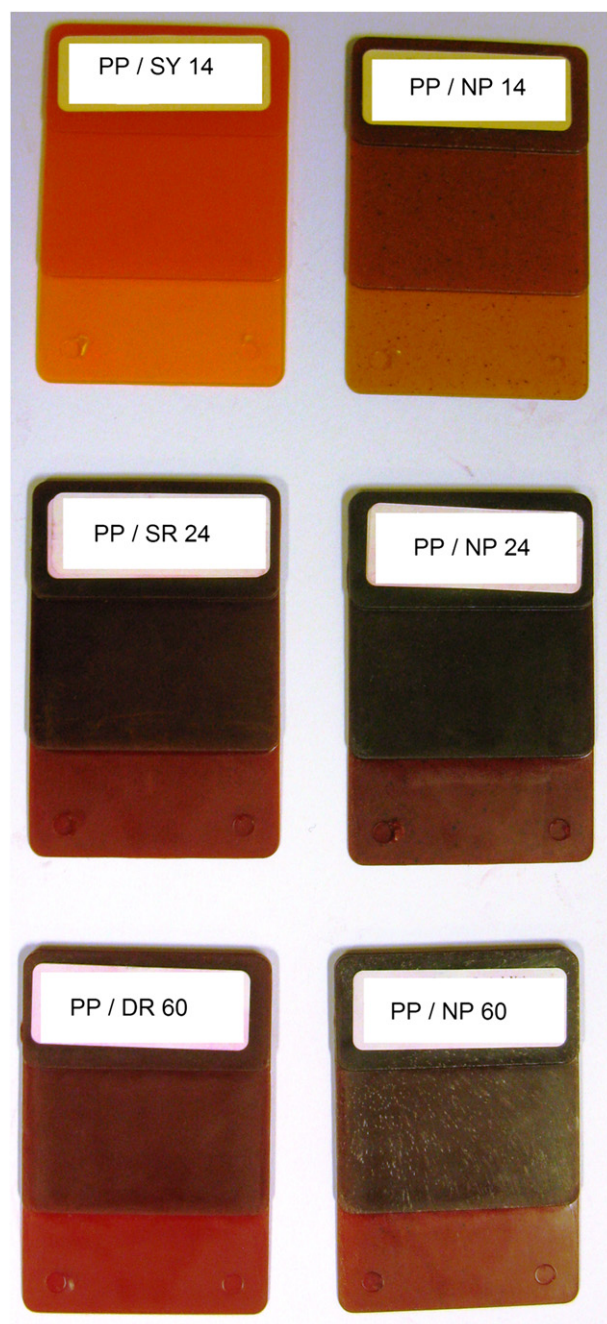
Fig. 5. Coloured polypropylene composites prepared by mixing the nanopigments and the corresponding original dyes.
